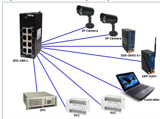
Connections of Ethernet devices
