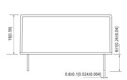
Case No.IRM02 Unit:mm[inch] Tolerance:±0.5[±0.02] unless otherwise specified
