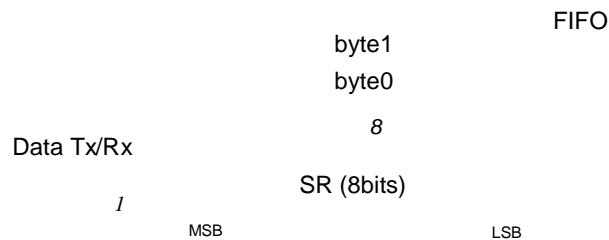
Figure 26. FIFO and Shift Register (SR)
