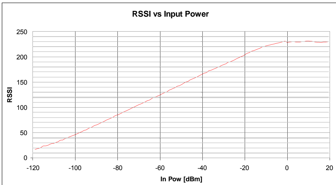
Figure 31. RSSI Value vs. Input Power
