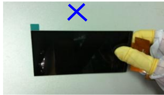
Please don't hold the surface of panel 请不要拿着面板的表面
