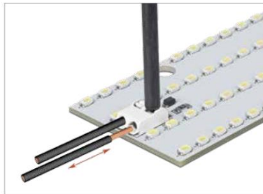
Inserting/removing fine-stranded conductors by lightly pressing on push-button (e.g., using a 206-860 operating tool).
