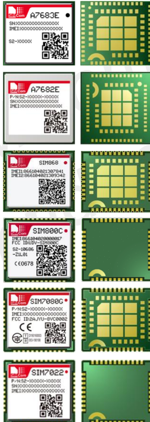
Figure 2: A7682E/A7683E/SIM800C/SIM868/SIM7080G/SIM7022 top and bottom view
