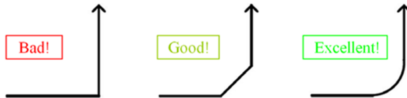
Figure 5-13: Examples of Turns in Trace Routing
