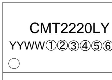
Figure 10. CMT2220LY Top Marking
