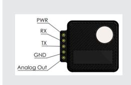
Analog voltage output ("Analog Out")
