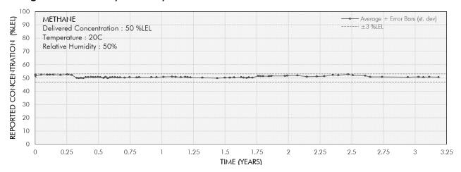
Average concentration reported to repeated exposures of 50 %LEL methane vs. time. Between exposures, all sensors were operated without airflow in ambient air. During exposures, all sensors were placed in an environmental chamber set at standard conditions (20  $^{\circ}$ C, 50 %RH) where gas was delivered from a cylinder. Accuracy remains within  $\pm 3$  %LEL over 3 years.
