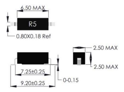
**RS-R5-S Reed Sensor PCB Layout drawing**
