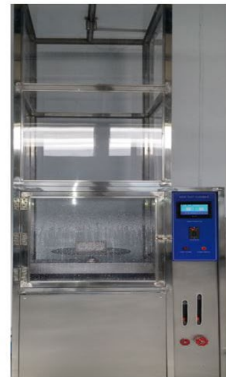
Testing under water jet
