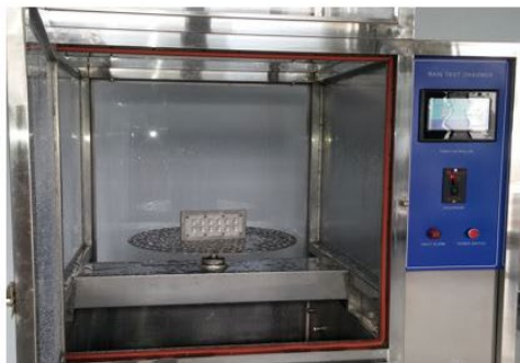
Testing under water jet
