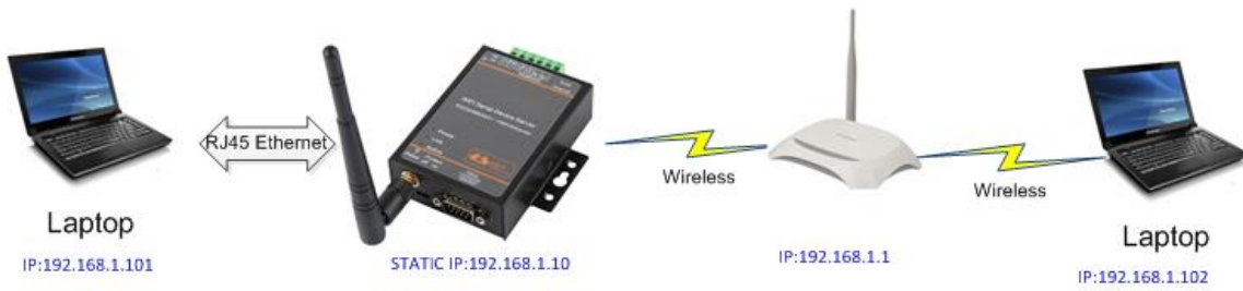
Figure 22. Ethernet Port Function(Bridge, reserved)
