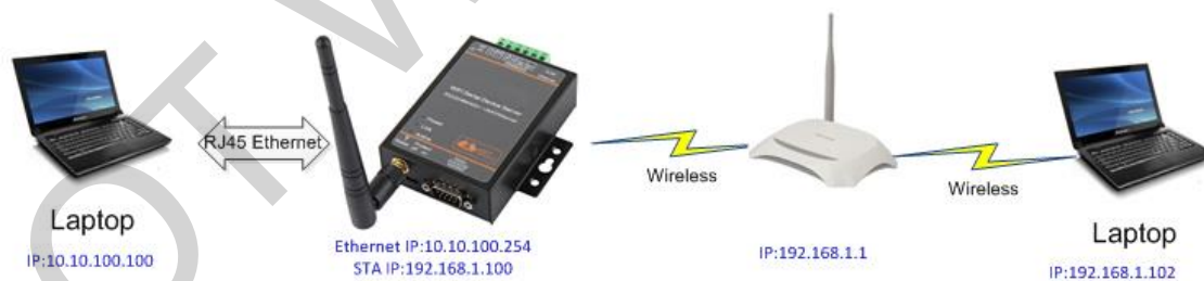
Figure 21. Ethernet Interface Function(Router)
