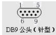
Figure 4. RS232 Pin Defination(Male/Needle Type)
