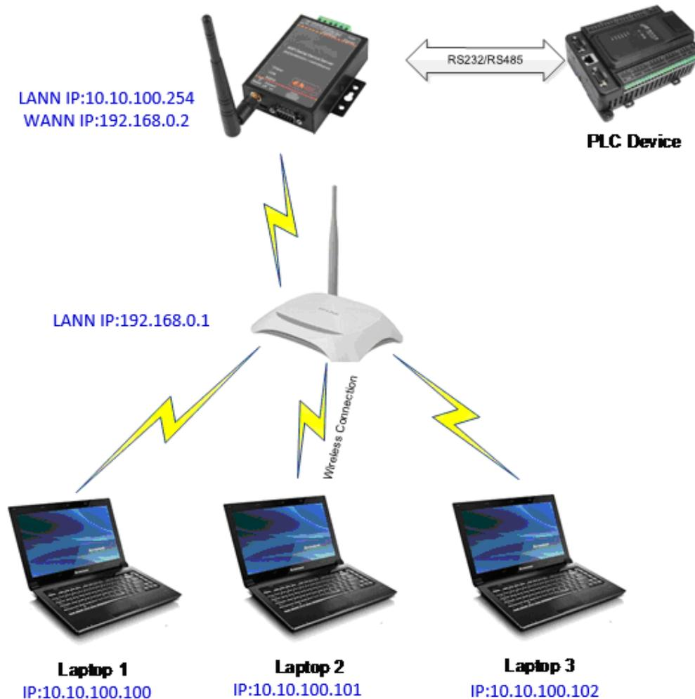
Step 1 : Factory parameter of HF2211 is AP mode. If need to modify to STA mode, it can adopt wireless direct connection with AP, Ethernet cable direct connection with PC and Ethernet cable direct connection with router.
