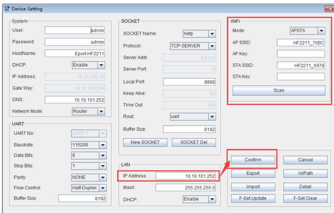
Step 7 : Restart after set successfully, PCWiFi connect to hotspot of class 2 device. Restart IOTService, it will show device information. In the meantime, HF2211 cascade connection is successful. "Router->class 1 device->class 2 device->terminal" are under the same network.
