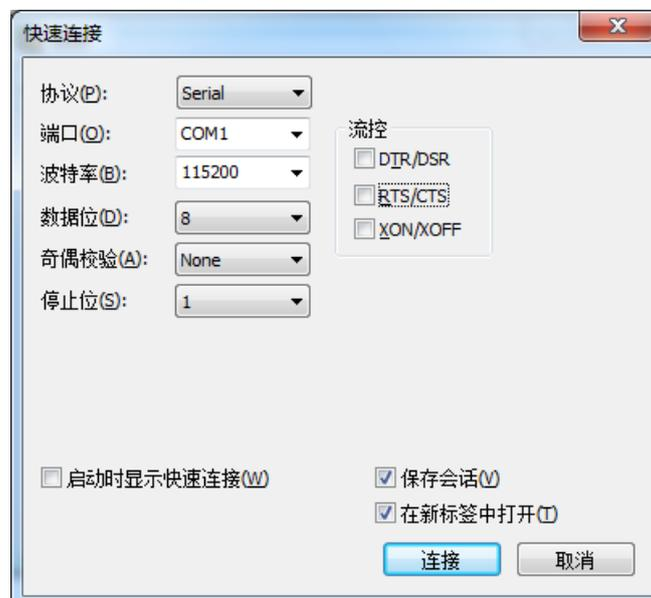
Notes: HF2211 the default serial data is as above and user can modify device working parameter by IOTService.
