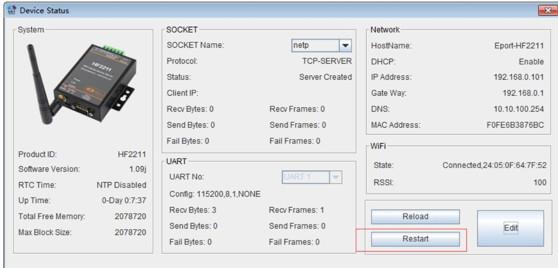
Step 4 : After restart, cable can be pulled out when the Link lights on. If device and terminal connect successfully, HF2211 can connect to the router as STA mode, and PC can connect the HF2211 AP hotspot. As a result, router, HF2211 and PC are under the same IP segment.
