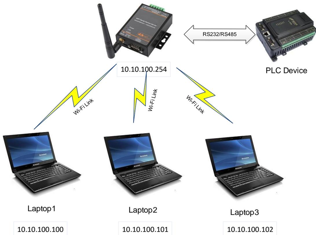
Step 1 : Before configure it as AP mode, AP SSID of AP should be understood first. The default is "HF2211\_+MAC(after 4 bits)". It can also search by command "show" in CLI command. Figure is as below:
