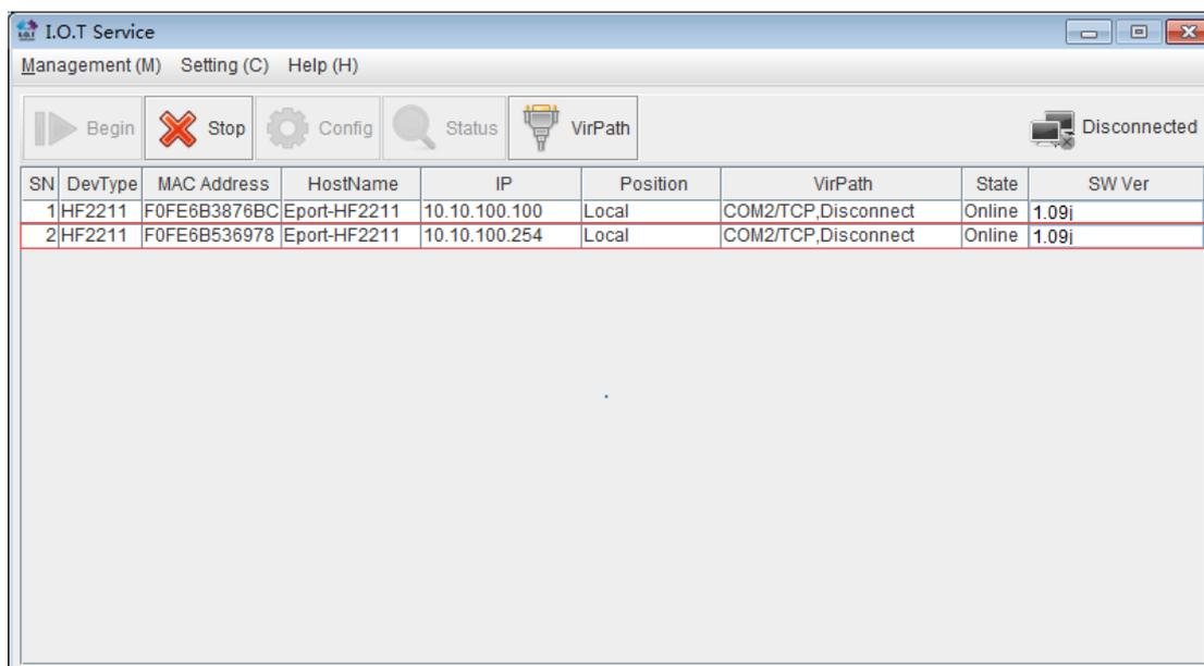
Step 6 : Repeat Setp 1 to Setp 4 to class 2 device. STA side connects to the class 1 hotspot. Besides, change IP address in LAN network. It will result that LAN address of class 2 device in the different network segment of WAN address of class 1.
