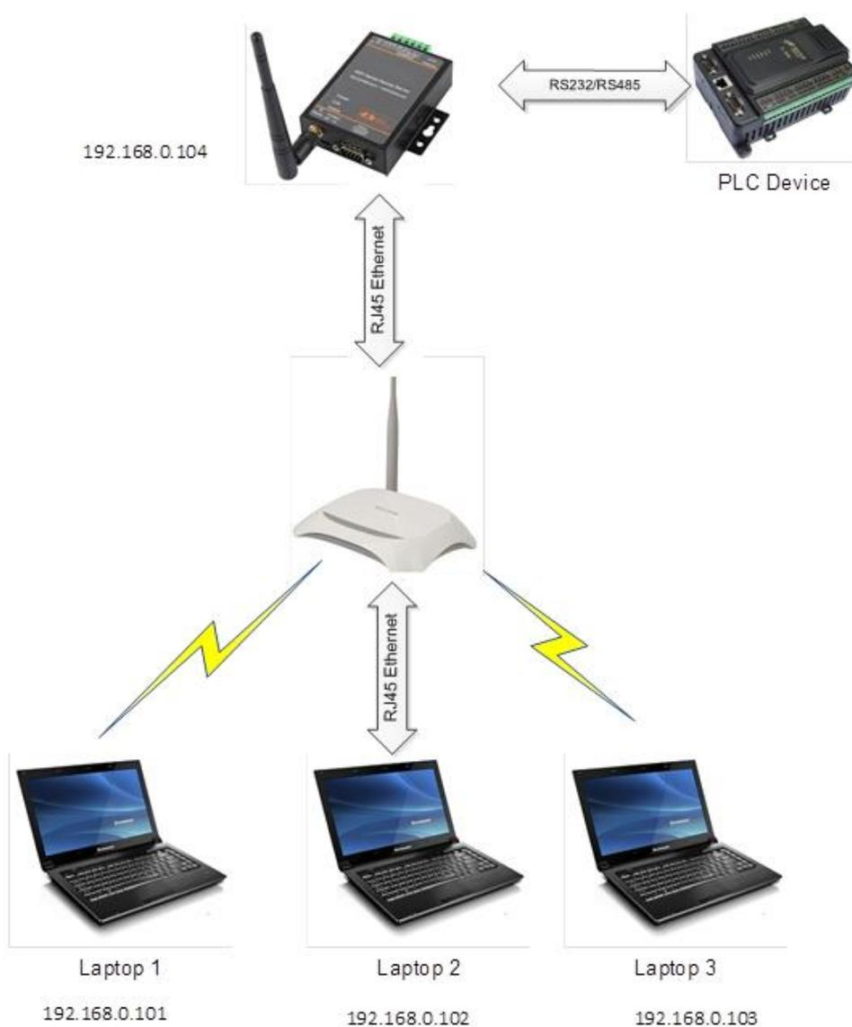
Step 1 : As above figure shows, HF2211 connect LAN port of router by Ethernet cable. PC is able to connect to the router to combian network by Ethernet or wireless.
