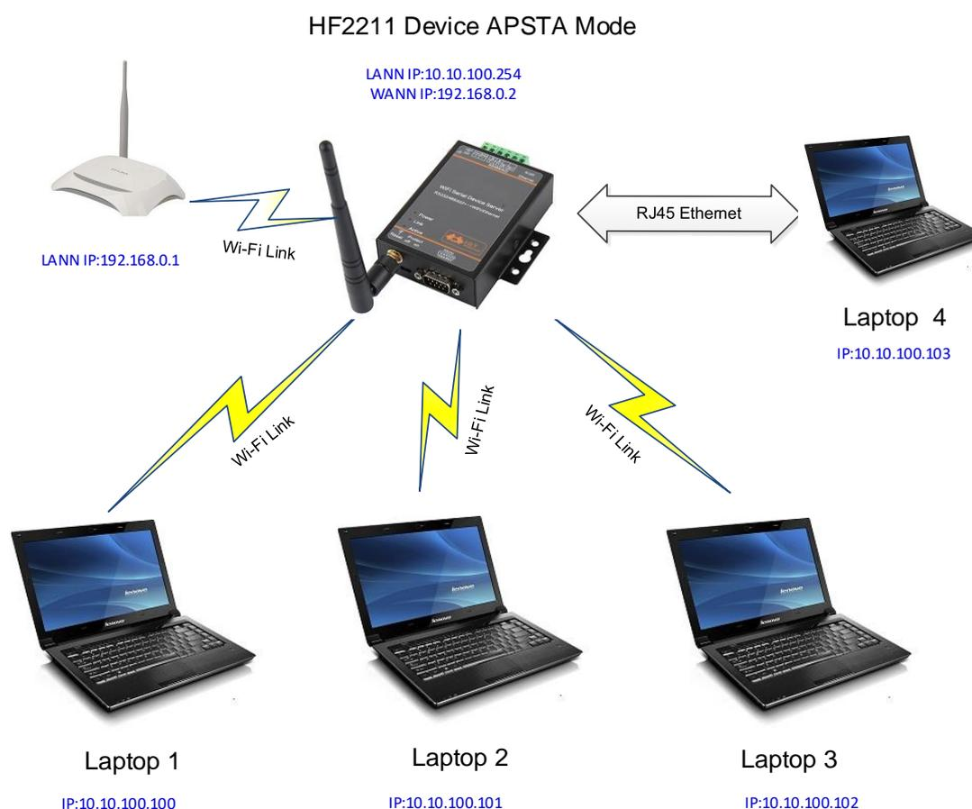
Step 1 : The default networking mode of HF2211 is AP. AP+STA mode can be changed by software or webpage.
