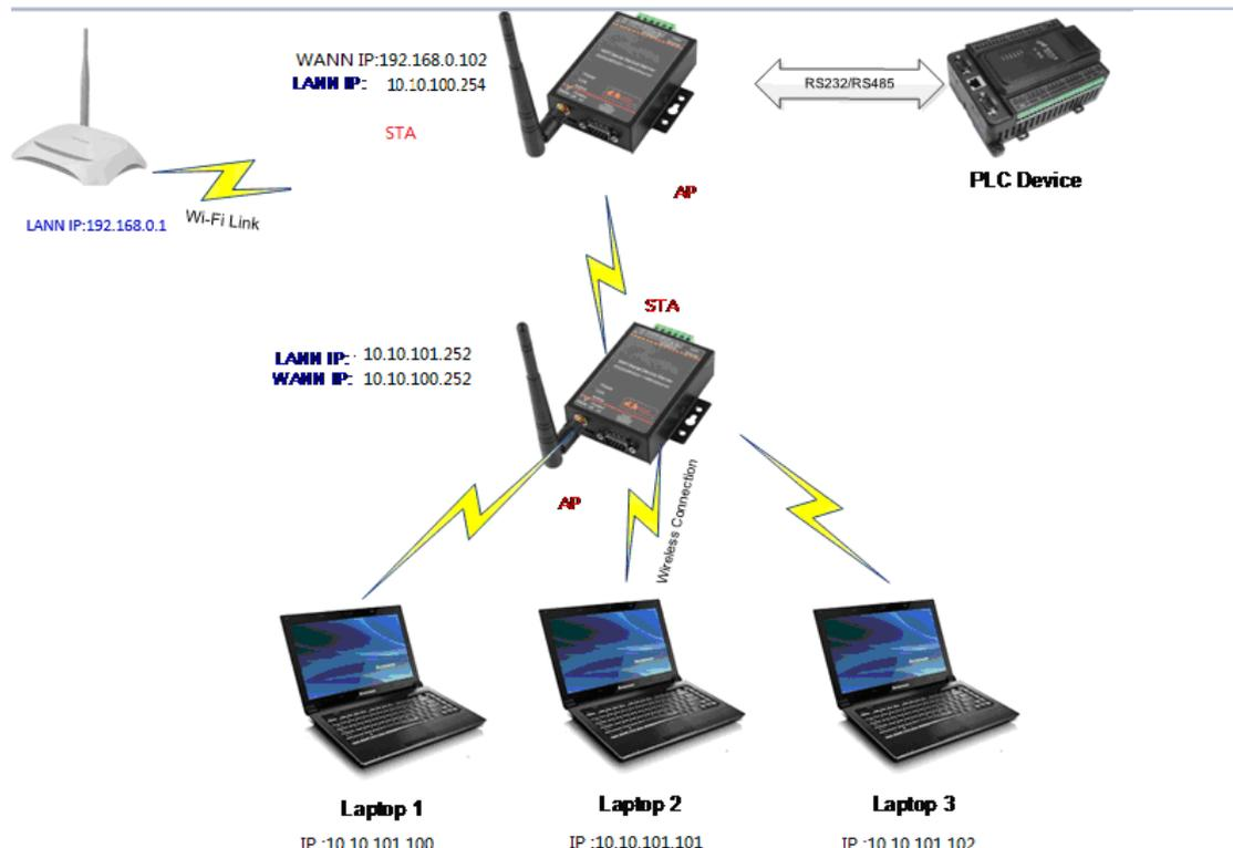
Step 1 : PC cable directly connect the Ethernet interface of first layer device(upper HF2211 in above figure). Open network and share center and forbid other connection method with only local connection.
